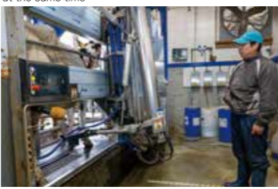
Automated cow milking machines automatically detect the presence of cows
